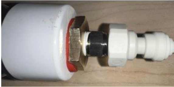
Figure 3 - Installed Bulkhead Connection on Modified Carbonator Bottle
